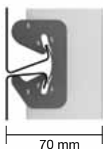
System depth with SE modular click rail
